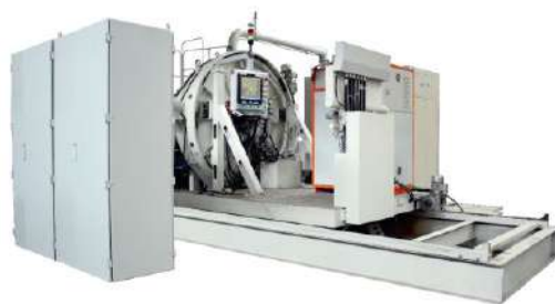
Figure 1. The «Granule» equipment works according to the PREP method.
